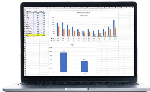
*Tord Beurling keeps a close eye on energy consumption. In the diagram, he compares what the new exhaust air heat pump consumes month by month compared to the old one.*
